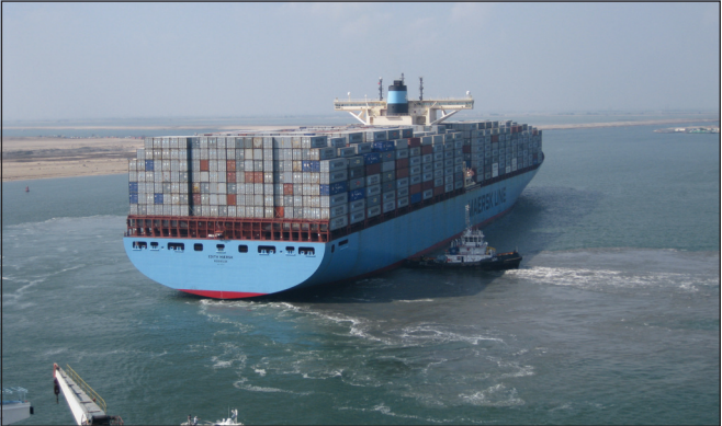
One of today’s leviathans, the 15,500 TEU EDITH MAERSK is 397m long and 56m wide and has a maximum draft of around 14.9m. The forthcoming Triple-Es measure 400m long, 59m wide and 73m deep and have a draft of 14.5m
